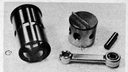
Heart of Blackhead is its piston and cylinder assembly. Piston of hi-strength Mahle alloy.
