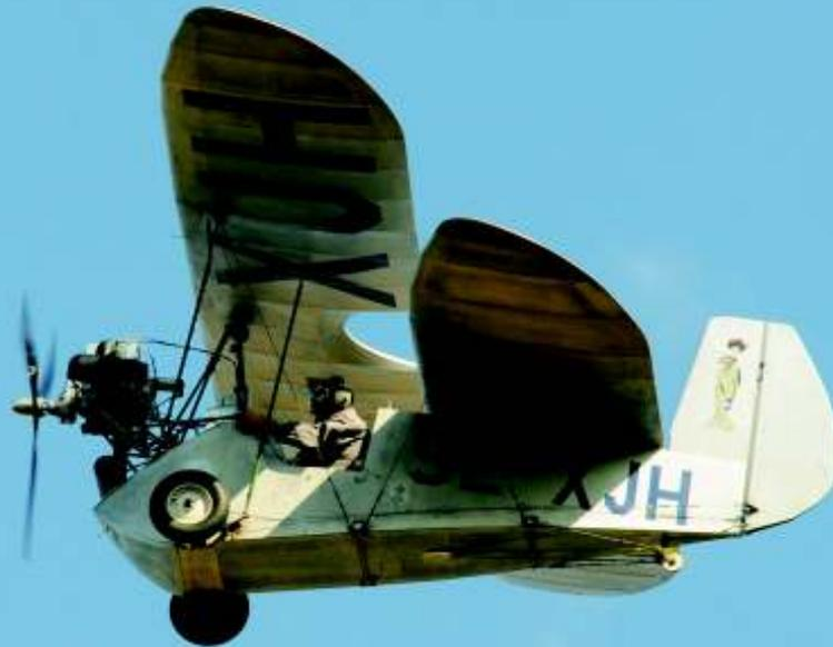
Flight tests of the Flying Flea type HM14 with HM290/3 wings, registration SE-XJH
