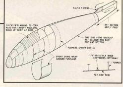
near the front are closer together to allow for the tighter compound curves. The end result is a plywood skinned fuselage, each segment butting up to the the next, smooth and ready for painting, much the same as on the real aircraft, with no unsiahtly sanded off high spots.
