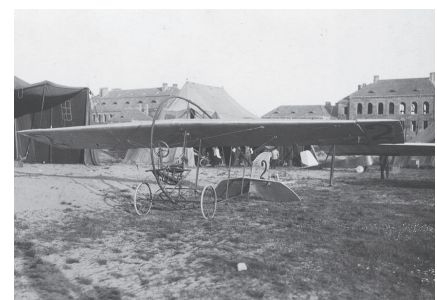
The early first version of the Bydgoszczanka (note position of the rudder). Photo: Skrzydlata Polska via www.piotrp.de
